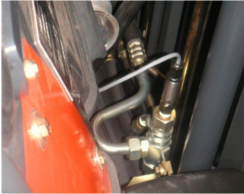
Typical Installation of the ED2 Series Pressure Transducer in Lifting Hydraulic Circuit
