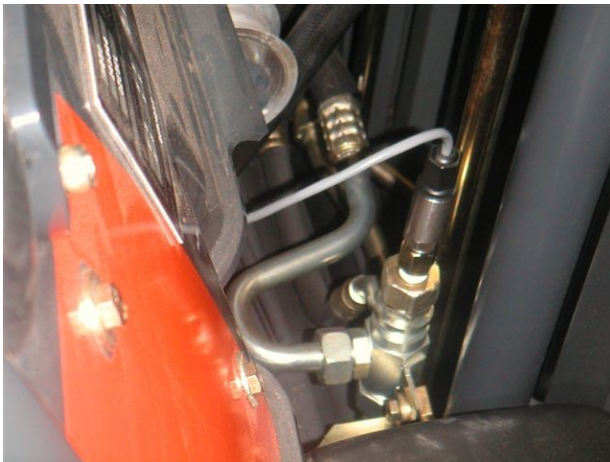
Typical Hydraulic Pressure Transducer Installation
