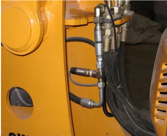
Typical Installation of the ED2 Series Pressure Transducer in Lifting Hydraulic Circuit
