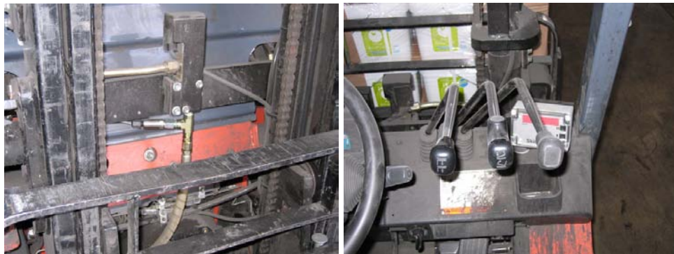
Example of the pressure transducer installation / digital indicator on Toyota forklifts with short mast
