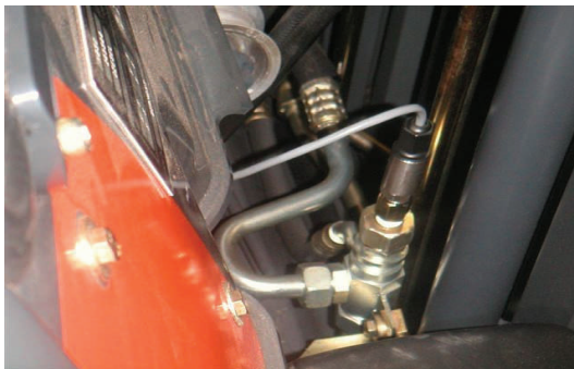
The installed system is calibrated automatically by lifting known load weight on the forks
