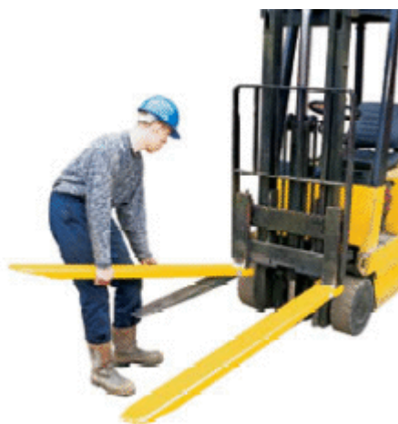
Example of re-calibrating of the system “zero weight” when extension forks are used
