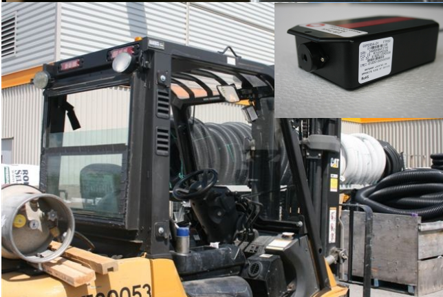
Typical installation location of the over speed monitor
